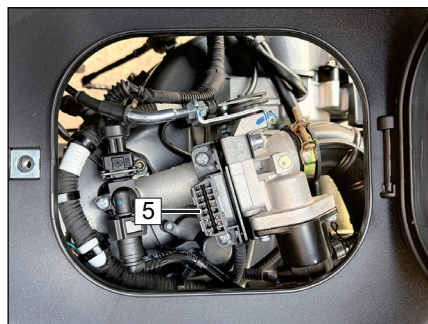
3. Fault diagnosis tester connector (5).
